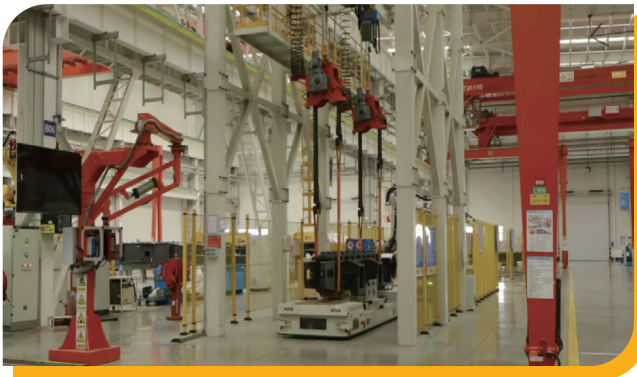
Automatic feeding of track rollers
