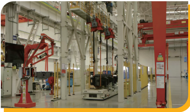
Automatic feeding of track rollers
