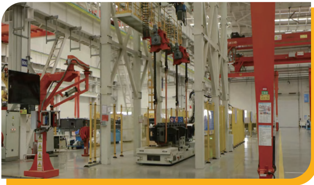
Strap-type Crawler Beam Turnover Machine
