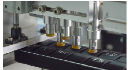
Panel buttons 1.2 million times reliability test
