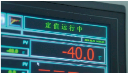
HMI display Low-temperature performance test under -40°C
