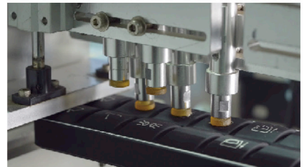
Panel buttons 1.2 million times reliability test
